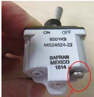
Screw Terminal MIL-DTL-3950 (5 in. lbs.)
